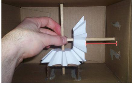
As with the first piece, you don't want to make the shelf's width (distance "A") larger than 1.25" (3.2cm) so as not to affect the gears' connection:
