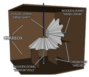
Now you'll need to find a box to use for the gearbox. Note that the above gear setup will fill a minimum space of a 4" (10cm) cube inside your gearbox (not 4in³, 4"x4"x4" = 64in³), so you'll want to give yourself some wiggle room in all directions, especially if you plan to add something in to weigh the box down. For reference, I chose a box sized 8.5" (21.5cm) wide X 5.5" (14cm) high X 7" (18cm) deep.
