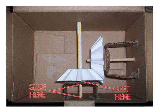
Now you'll want to glue the support pole dowel in place. It will attach to the bottom of the box and optionally the shelf (for extra stability), but <u>not</u> to the straw drive shaft (it should still spin independently, as shown above). Once dry, you should finally be able to turn the handle and have it spin the drive shaft.
