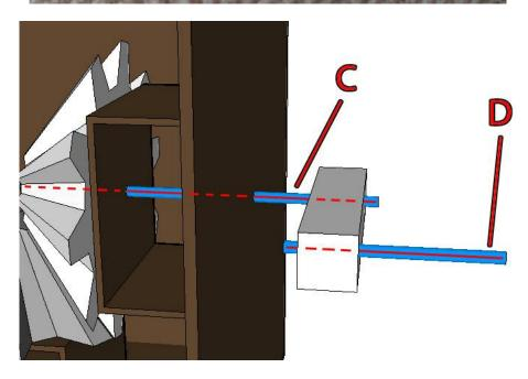
To find the length of piece "C", feed a dowel through the top hole of the box. You want to measure the distance "X" between this pole and the wall where the hand crank will be:
