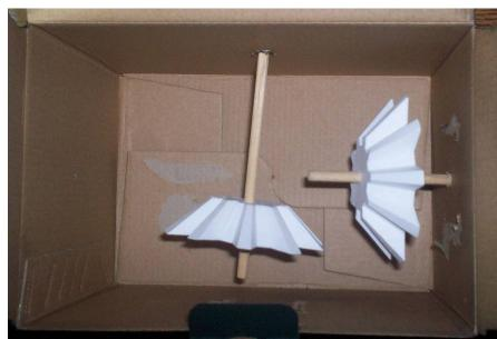
Get a ruler or tape measure handy. Hold the gears by their shafts, level the dowels, and push the gears together tightly to mimic how it will look completed.
