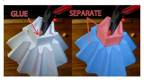
I recommend hot glue for attaching this section, as it's less likely to leak through the tube's hole and accidentally glue the two sections together.
