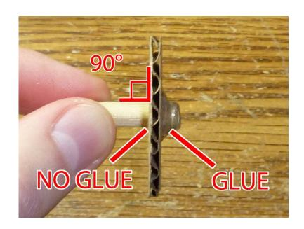
Once dry, take one and feed it through the hole you made in your first gear, so the large portion of the dowel is poking outside the gear, and the disc is inside:
