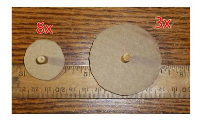
You want to glue a dowel through the center of each disc, leaving roughly 1/4 of the total length hanging out on one side. I would recommend only gluing the disc on the side with the short amount of dowel. Try to align the discs as close to perpendicular as possible:
