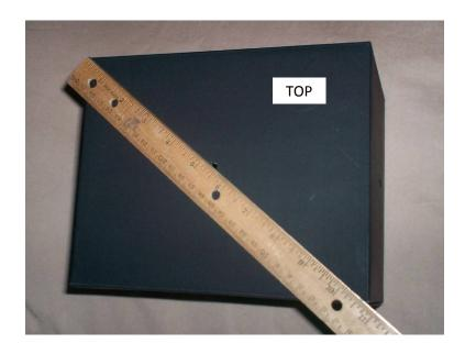
For the hand crank hole (only on one side of the box, not both sides), you'll want the hole to be horizontally centered, and vertically close to the top of the box while still leaving the gear space to spin. You can center it vertically if you want, but putting it closer to the top will give you more stability in the drive shaft's pole when we add it in later:
