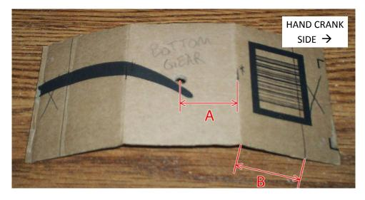
The width of the piece (distance "A") should be NO LONGER than 1.25" (3.2cm) so it does not interfere with the gears. It can extend as far as you like in the opposite direction. The dowel should fit the hole very tightly (the straw will NOT be going through it).
